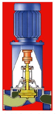
column through which flows the discharge fluid. The intermediate bearings are lubricated by the fluid as it passes up the column.
