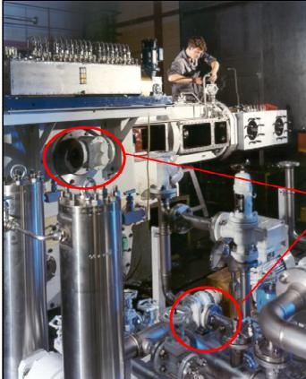
High pressure reciprocating compressor fitted with a crankshaft driven 3" Albany gear pump. A motor driven Albany API 676 pump gives pre and post lube service.
